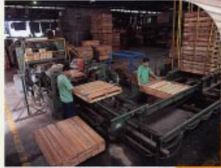
Automated Pallet Assembly Line
